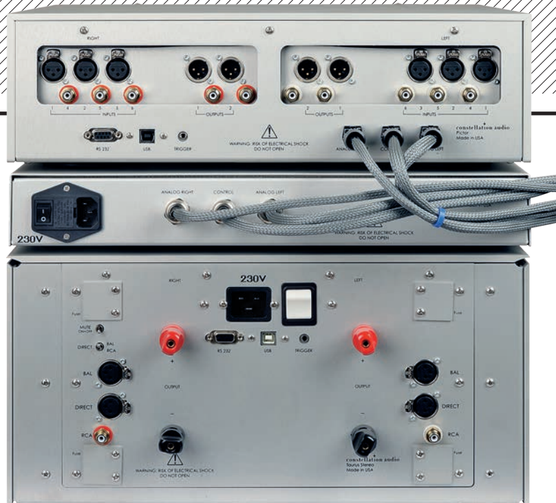
ABOVE: Pictor preamp [top] has an outboard PSU [middle], three balanced (XLR) and single-ended (RCA) ins with pairs of XLR/RCA outs. USB port is for control/updates. The Taurus [bottom] has 4mm speaker outlets, RCA and full/low (Direct) gain XLR ins
